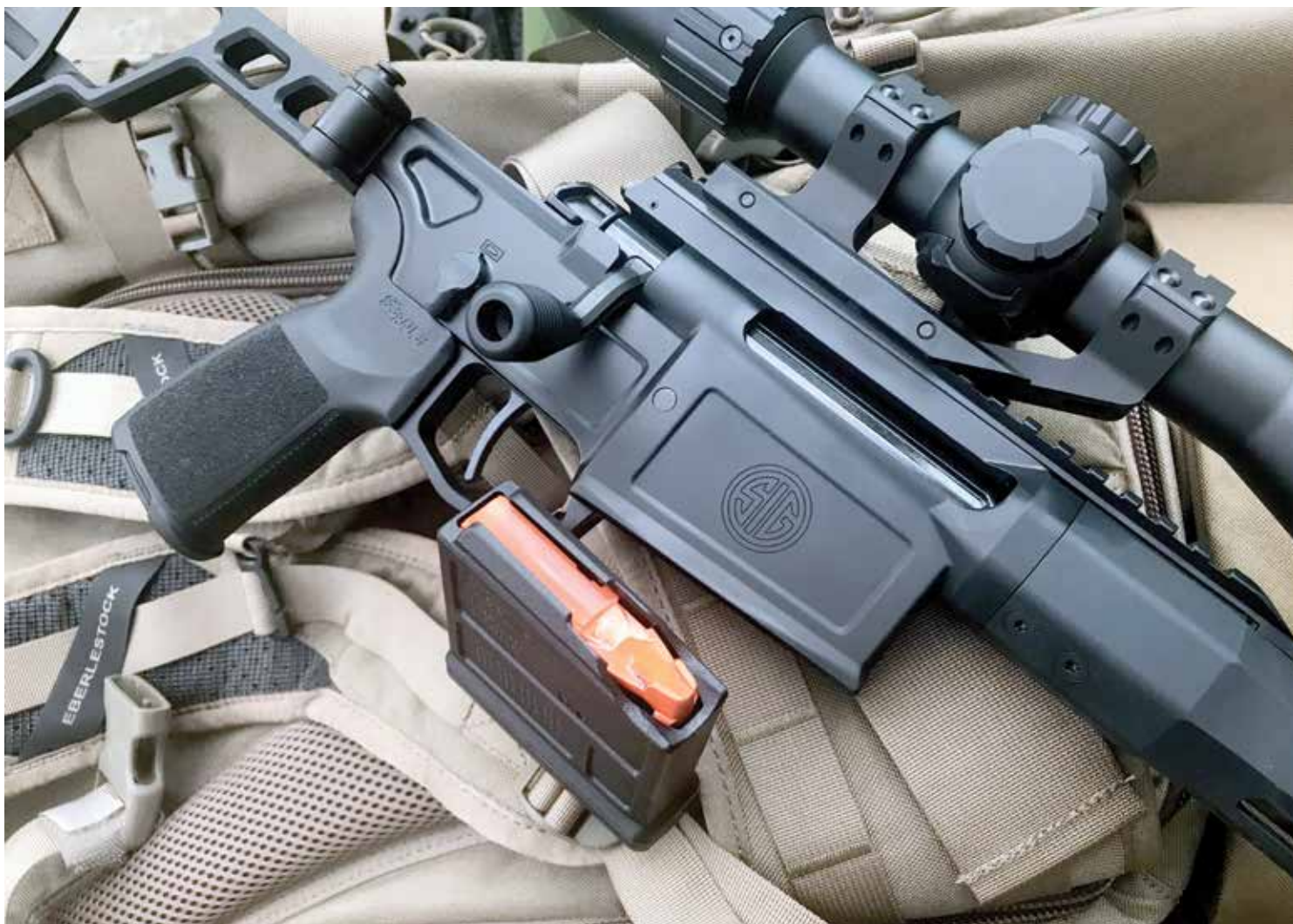
The CROSS feeds from standard AICS-pattern magazines with a Magpul 5-rounder arriving with the rifle. The magazine has proprietary sled follower for optimized single-round loading through the ejection port.
