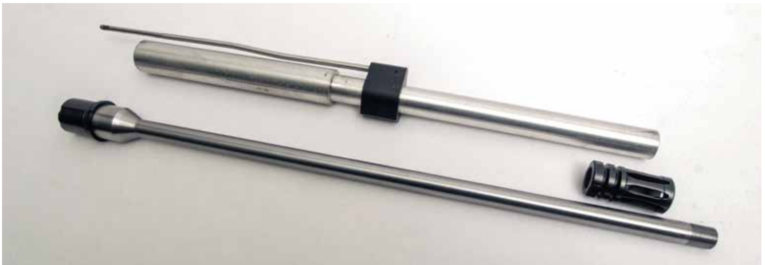
M4 cryogenically-treated barrel and ZK magnesium sleeve with gas block, before assembly of sleeve over the barrel.
