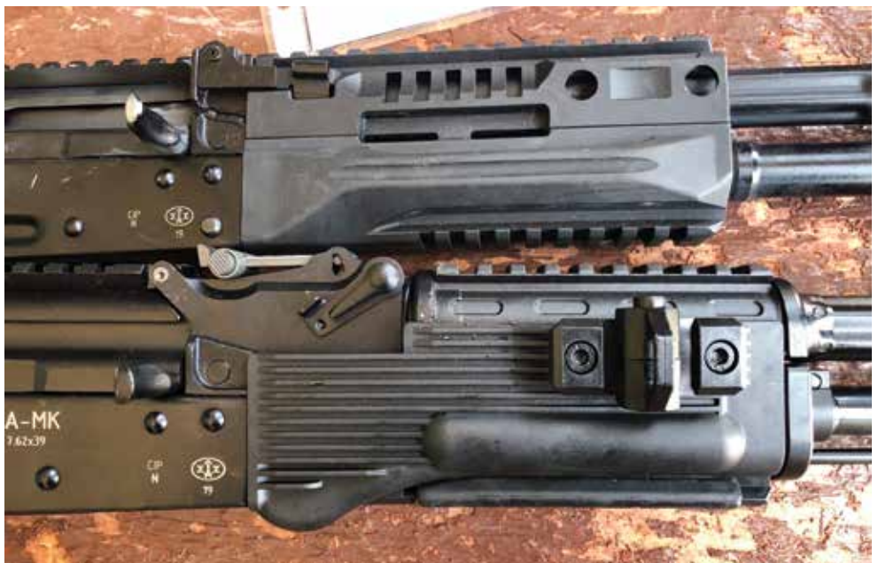
Handguards, AK-200 uses the same interface as all previous AK generations, allowing it to use previously-available rail systems.
