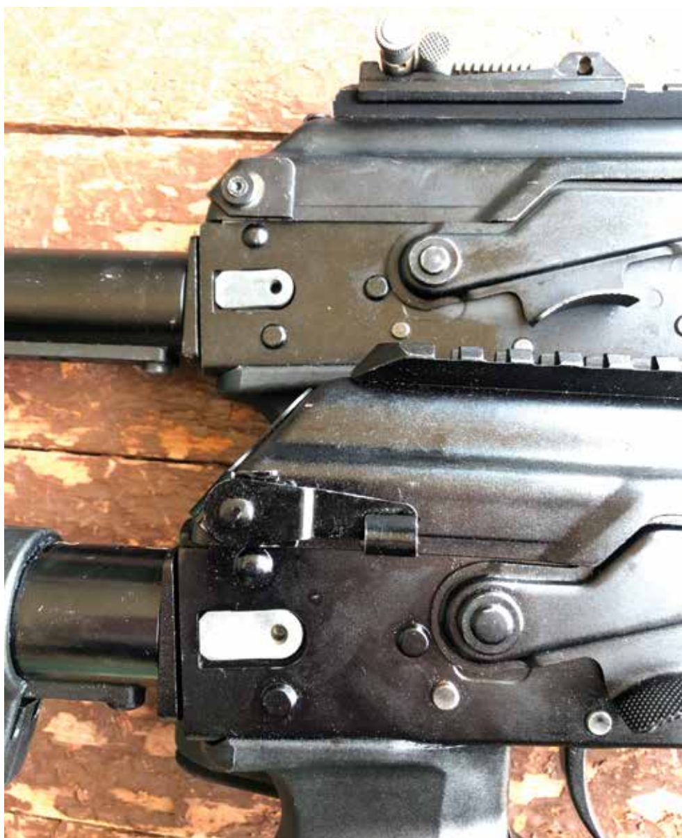
View of the rear of the receivers and top cover. Note an extra rivet below the safety, this is connected to a device which disables the trigger when the stock is folded (for Russian civilian firearm overall length regulations).
