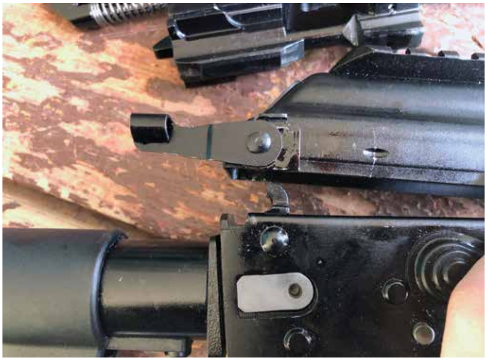
AK-200 rear trunnion and top cover interface. Note that AK-12, 15 and 200 series all use the same rear trunnion.
